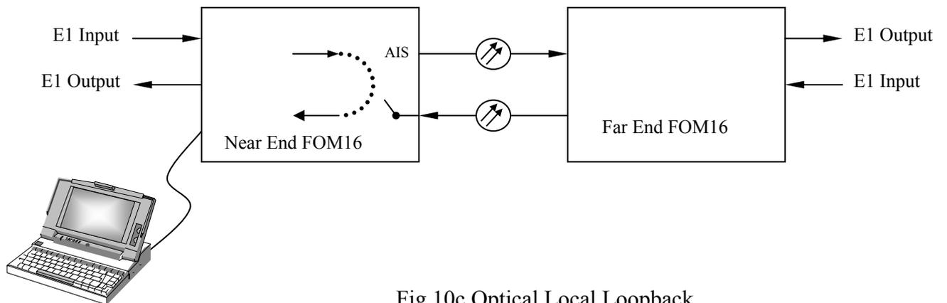
Fig.10c Optical Local Loopback
